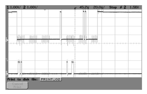
Figure 3.22: ADC DIN and DOUT with analog input signal
