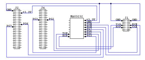
Figure 5.12: Wiring of the MAX3232 on the RCM3100 evaluation board
