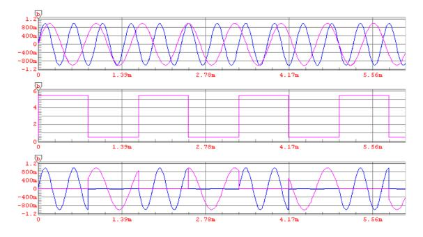
Figure 5.9: 1300/2100Hz Frequency Shift Keying
