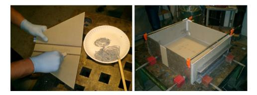
Figure 2.1: Milled honeycomb getting bonded and put in place
