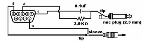
Figure 5.13: Wiring suggestion for ICOM radios
