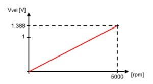
Figure 3.23: Velocity monitor out vs. motor revolution
