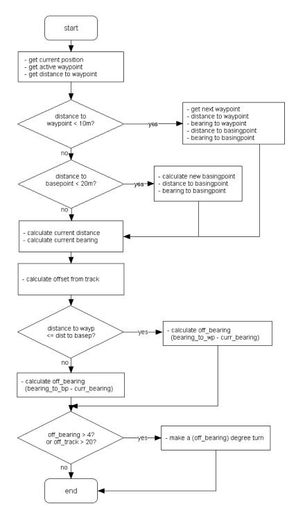
Figure 3.8: Flowchart for basic navigation algorithm
