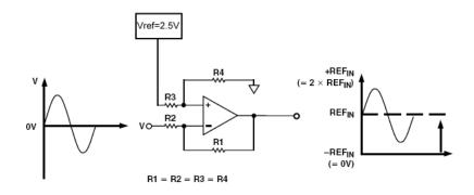
Figure 3.21: Circuit to bias bipolar signals about Vref
