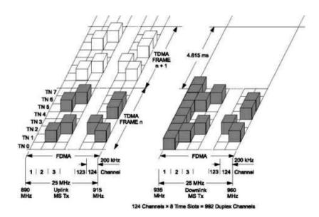
Figure 5.2: FDMA versus TDMA
