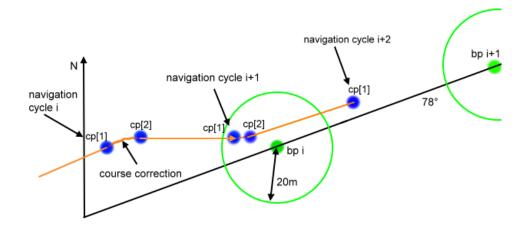
Figure 3.14: Basing point generating example (drawing)
