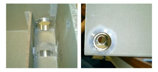
Figure 2.4: Top view of the support tube mounts and view along one of the axles
