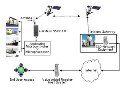
Figure 5.1: Example for an IRIDIUM modem application
