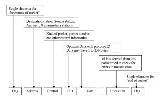
Figure 5.18: Structure of KPC3plus data packets
