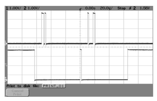
Figure 3.18: Sample SPI communication on serial port B
