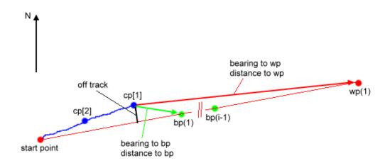
Figure 3.2: Visualization of most important terms for GPS navigation
