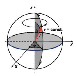
Figure 3.16: Spherical coordinates
