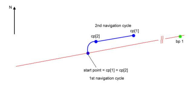
Figure 3.10: Startup procedure 1 with Cool Robot pointing north
