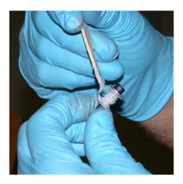
Figure 2.2: Inserts with epoxy
