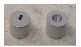
Figure 2.5: The aluminum shaft collars
