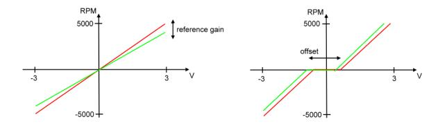
Figure 4.4: Motor revolutions vs. input voltage
