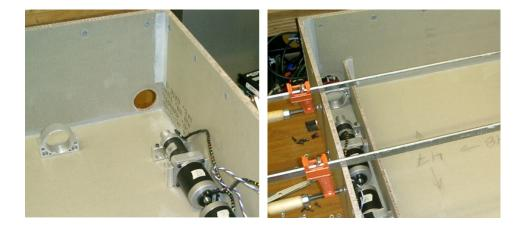
Figure 2.3: Chassis without and with partition wall
