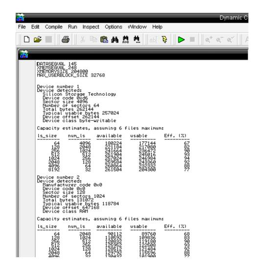
Figure 6.3: Screen shot of FS2 sample program showing specifications of the Flash memory
