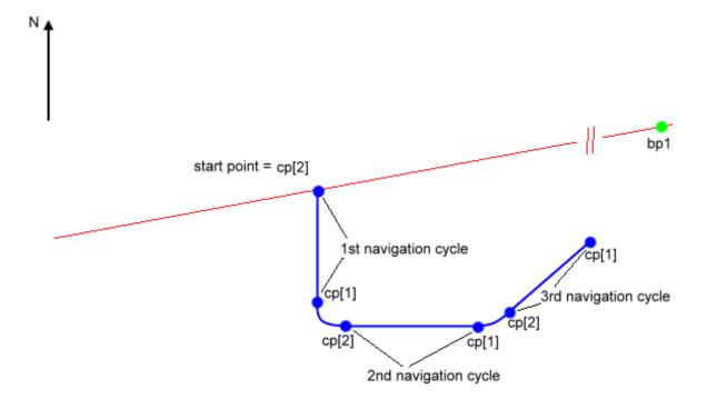
Figure 3.12: Startup procedure 2 with Cool Robot pointing south
