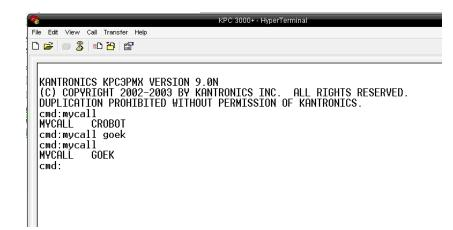
Figure 5.15: MYCALL command using Hyperterminal
