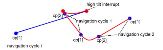
Figure 3.24: High tilt angle interrupt handling sample
