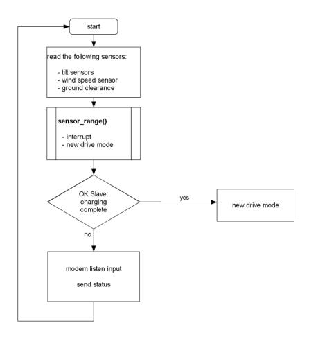
Figure 4.8: Drive mode charge cycle
