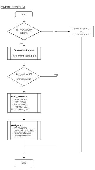
Figure 4.5: Flowchart of drive mode waypoint following at full speed
