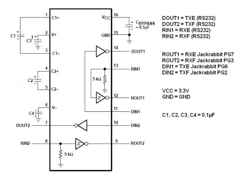
Figure 5.11: Pinouts MAX3232 RS232 line driver/receiver
