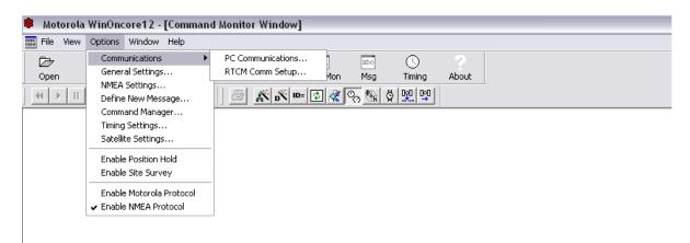
Figure 3.4: Options to initialize the GPS unit to output NMEA data
