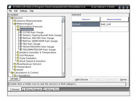
Figure 6.5: Screen shot of "Short Cut" second step: choosing sensors
