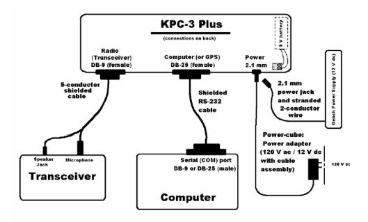
Figure 5.10: Basic wiring of the KPC3plus radio modem
