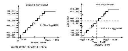
Figure 3.20: Straight binary vs. twos complement output format
