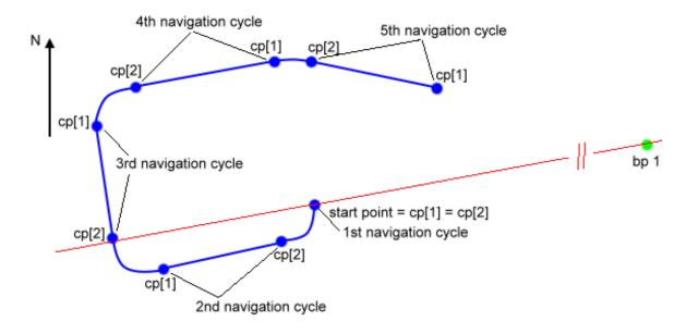
Figure 3.11: Startup procedure 1 with Cool Robot pointing south
