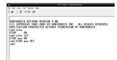
Figure 5.16: ECHO ON/OFF command using Hyperterminal
