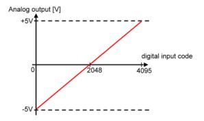
Figure 4.3: Voltage output vs. digital input
