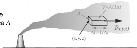
Figure 4.A.1 Flux, \vec{J} , is a vector quantity whose value varies with position (x, y, z) . The contaminant flux vector points in the direction of transport, and its magnitude is the quantity transported (usually mass or moles) per area per time.
