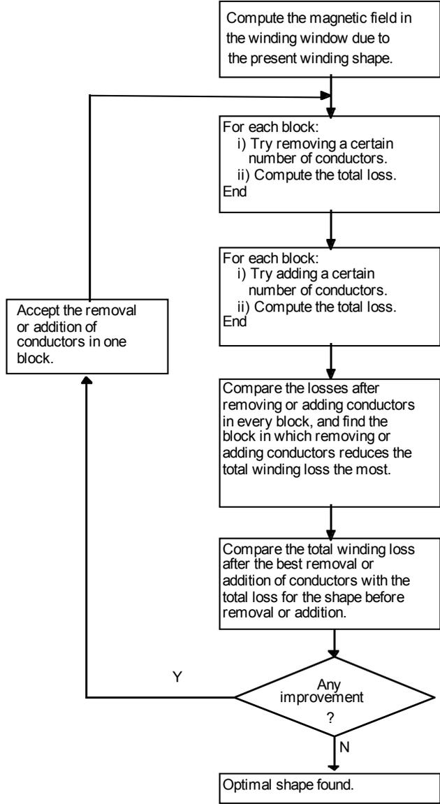
Fig. 3. Flow chart of the COOS optimization algorithm.
